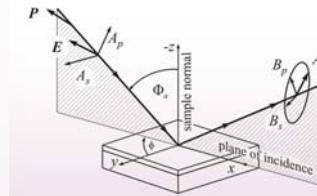
The 4x4 real-valued Mueller matrix connects the incident and emergent Stokes vector components, which are linear combinations of different polarization states.
