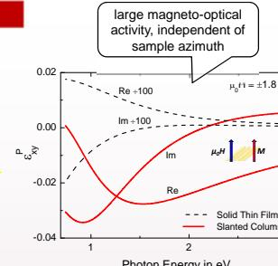
At 1.8 T all domains are parallel to the external magnetic field. Only an azimuthally independent  $\varepsilon^P$  is necessary to model magneto-optic coupling.
