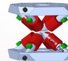
An octupole vector magnet allows for generalized ellipsometry measurements at arbitrary magnetic field orientations.
